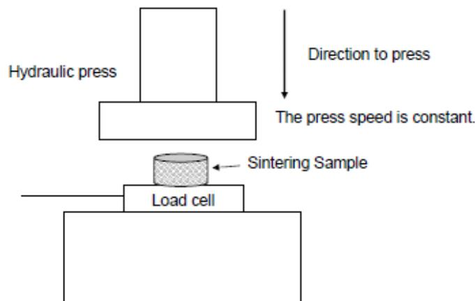
**Figure 4:** Press machine scheme
