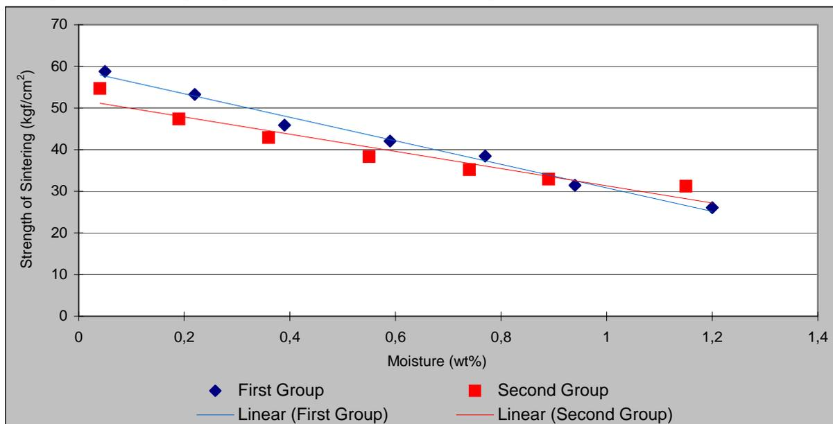
**Figure 5:** Relationship between sintering intensity and moisture
