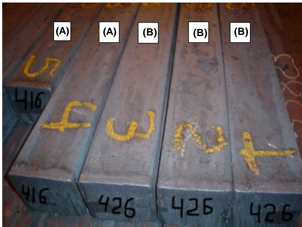
Fig. 4 – Surface of billets cast with LCB 416 (A) and LCB 426 (B)
